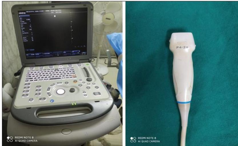
**Fig 3(a):** Portable MINDRAY Echocardiogram Mechine (b) Transducer Probe
